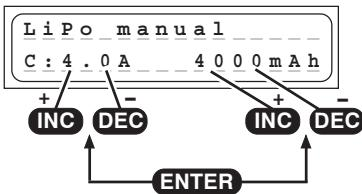
This program charges the battery using the capacity (charge current) which you set.
