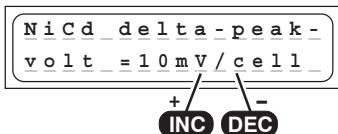
The automatic charge termination circuit (battery full detection) works on the proven Delta Peak principle (also known as the Delta-V process), which is already in use in millions of chargers.
