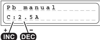
In this program you can set the maximum permissible charge current using the INC / DEC buttons, but only **before** you connect the lead-acid battery for charging. This setting only determines the top limit which the charger is permitted to feed to the battery.
