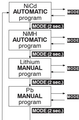
In the interests of clarity, the charge and set-up facilities of the ULTRAMAT 16 are divided into four logical program groups. A separate program group is provided for each of the different battery types: **Nickel-Cadmium**, **Nickel-Metal-Hydride**, **Lithium-Ion / Lithium-Polymer / LiFePO<sub>4</sub> (LiFe)** and **Pb** (lead-acid) batteries.
