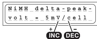
It is possible to adjust the trigger voltage (in mV per cell!) of the automatic termination circuit for Ni-MH batteries.
