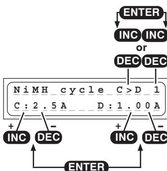
This program is designed to optimise the capacity of a battery, and balance the state of its cells.
