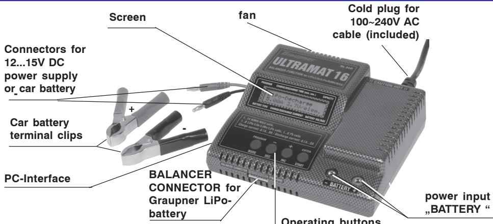
All the charger's functions are controlled by means of just four buttons.
