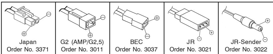
Be sure to use genuine charge leads fitted with cable of adequate conductor cross-section.
