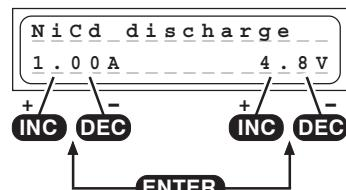
The typical purpose of this program is to determine the residual capacity of a transmitter, receiver or drive battery, or to discharge the pack to a defined level.
