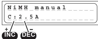
Select this program when you simply wish to recharge a battery using the set charge current. You can adjust the charge current using the INC / DEC buttons, but only **before** you connect the pack for charging. The range available is 0.1 A to 8 A.
