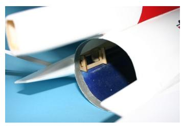
Before you glue the servo brackets in place, trial fit your servo (min. 2kg torque with metal gear), 2 micro servos are necessary. Also pre-drill the holes for the servo fastening screws. Also make the pushrods first with a z-bend at each end. How to make this z-bend is explained on page 7.
