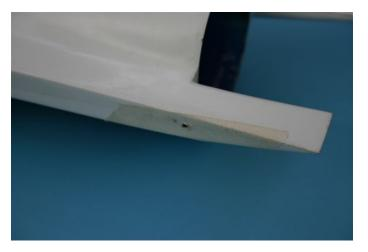
Put tape around the root of the elevon and the side of the fuselage.
