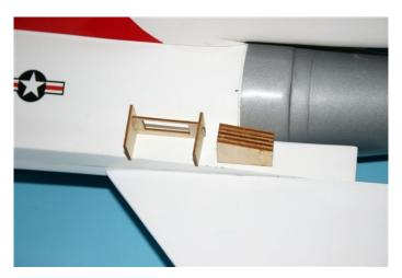
Assemble the servo-brackets, there's a high-side and a low side on the bracket, so the sides are different. The small edge on the Servo tray should be on top. The bottoms of the sides are almost square.
