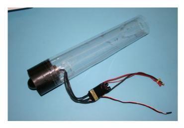
Read the installation instruction from your fan-unit first. Install motor and ESC first. You can either install the ESC inside the thrust tube or outside. We recommend to places the ESC behind the motor inside the thrust tube. Trim off the mounting tabs from the fan-shroud otherwise the fan unit will not fit. You can use our already made fiberglass thrust tube see top left picture. Tape the thrust-tube to the fan-unit.
