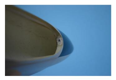
Tape the canopy frame to the fuselage so that all sides are flush.
