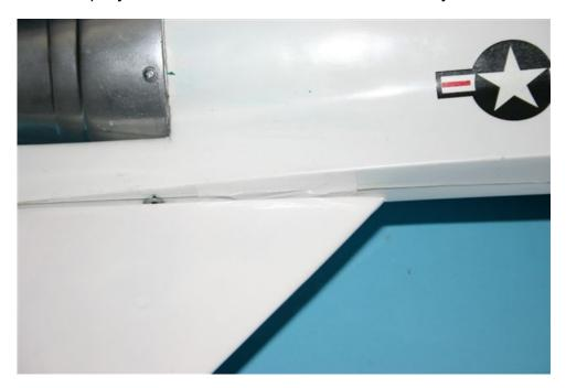
The Gap over the servo bracket can be covered with white vinyl decal or a piece of white iron on covering.
