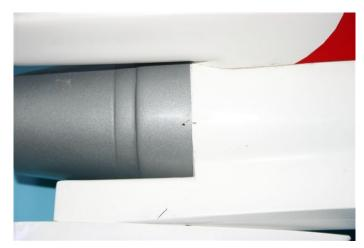
Mark the location of the plywood pieces a marker in front of the back ring as you need to drill holes through the exhaust-cone and the ply wood pieces. So after you marked the location of the plywood pieces. Slide the exhaust-cone over the back-ring of the fuselage, and drill 4 1.5mm holes through the exhaust cone and the plywood pieces.
