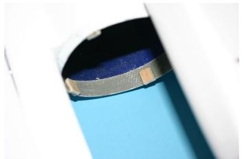
Take out the 4 small rectangular pieces from the bag with hardware and glue them in the back-ring of the fuselage with 5 minute epoxy. Look at the above picture.
