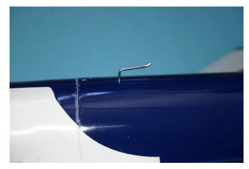
Behind the joint a plywood block is glued in the fuselage. No drill a 2 mm hole approximately 25 mm behind the joint, this hole is for the bungee hook. Glue the bungee hook in the fuselage with 5 minute epoxy
