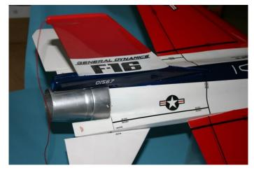
Battery location, next picture you see the receiver antenna coming out the top end of the fin. You need to drill a hole here.
