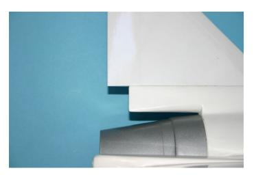
Put the main wings on some brackets and make sure the main wings are level. The elevons should have a +/- 10 degrees negative angle. Both tips of the elevons should have the same height from the building board.
