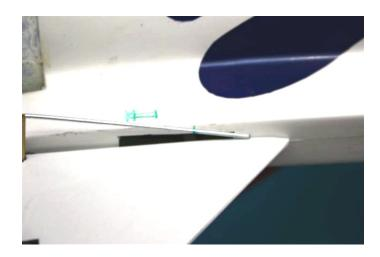
Mark the position of the servo pinion (servo control-horn) on the fuselage. Now transfer this position with a marker on the pushrod (elevon in app 3 degrees up position.)
