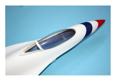
Attention: Before you trim the edges from the clear abs canopy trial fit it several times and assure that it has a good seat (fit). Make sure is does not put stress on the canopy frame.
