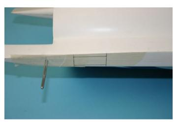
Mark the position for the Pivot-rod (2 3 mm steel rods one for each side) 62 mm from the end of the fuselage. Drill a little oversized hole in the middle at the marked location. We recommend a 4 mm hole. Wait before you glue the pivot rod in place.
