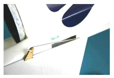
Glue the servo brackets in place with 5 minute epoxy. Wait till the glue is cured. Stick the Elevon on the pivot rod (with the final installation of the Elevon us should add the supplied Washer to act as a spacer between the elevon and fuselage.) The plywood control should not be glued yet in the elevon.
