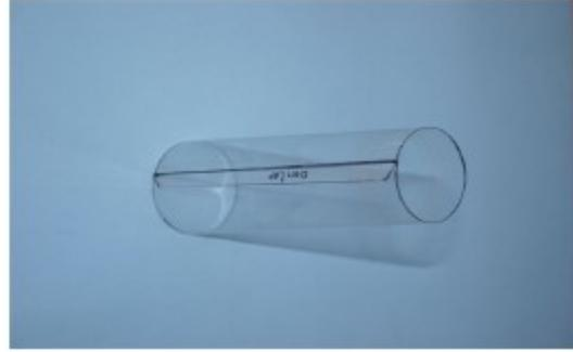
Cut out the unrolled surface for both trust tubes. Put the overlap area inside. Roll the pvc to a tube and apply outside adhesive tape. The Edge should match the innerline of the overlap area. Now you have a perfect conical trust tube.
