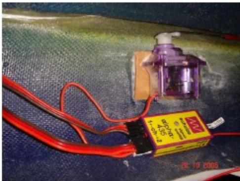
On the left picture you see the 4 channel micro receiver attached next to the servo with Velcro. You can also tape the servo wires to the top. So the wires will not be in the way when you install the ducted fan.
