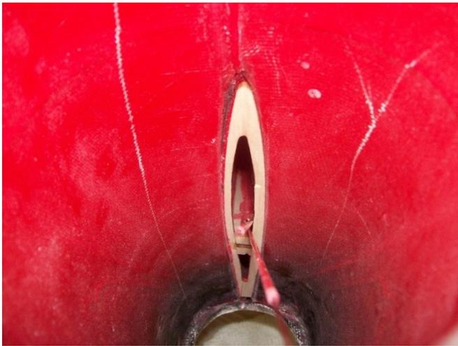
Now repeat these steps on the other side of the vertical stabilizer. (There is one control rod for either elevator half.)
