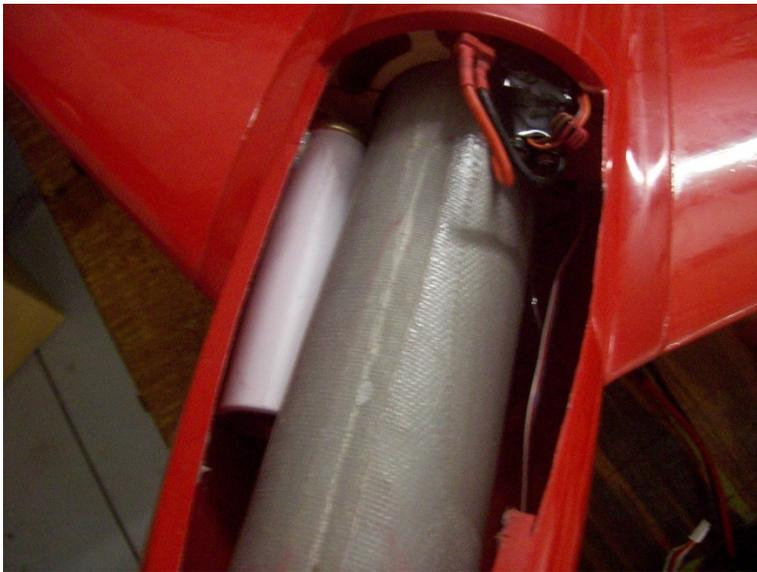
Next we need to mount the fan assembly. This setup is very easy to install. First make up your exhaust tube out of the included mylar clear sheet. Then tape the mylar tube to the rear of the fan. Now we can insert the fan and exhaust tube assembly into the jet. Next simply use a few drops of hot glue on the fan housing to secure it to the intake ducting...
