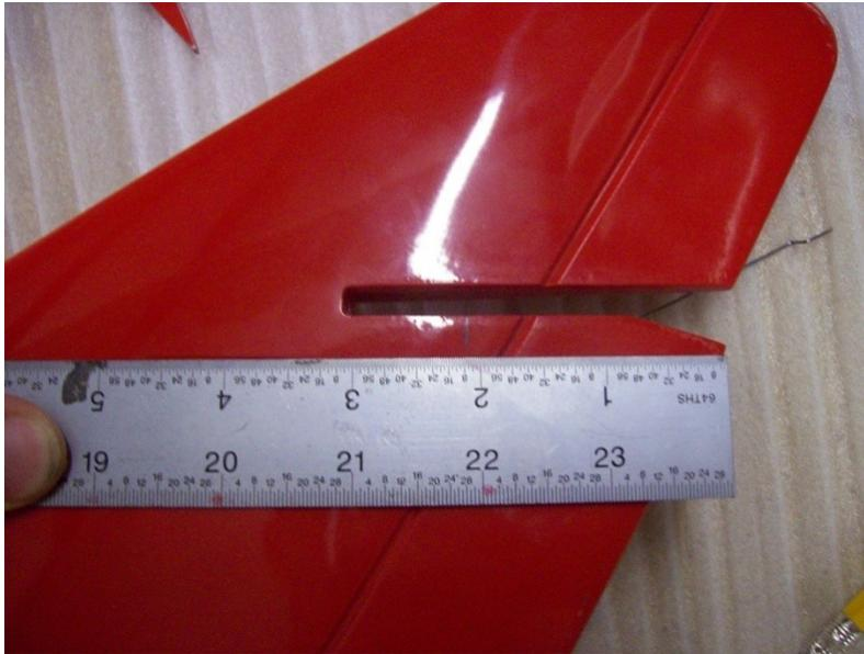
The next measurement is  $\frac{5}{8}$ " down from the horizontal stabilizer saddle on the vertical stabilizer and put a mark. (see picture below).
