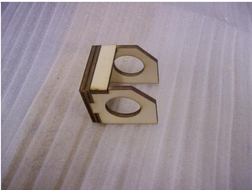
From this point the nose gear retract mount can be mounted permanently with epoxy and the nose retract can be screwed on with four screws.
