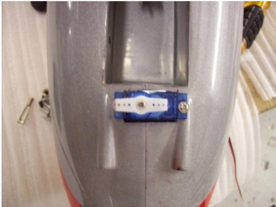
Now that the steerable nose wheel servo is in place we need to connect the linkage. First begin by installing your control linkage. Next use two pieces of scrap 1/8" plywood 1" back from the servo on either side of the retract recess. These plywood pieces keep the retract linkage from getting tangled around the strut when the nose wheel is retracted. See pic below.
