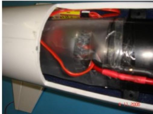
Before you install the fan-unit you must add some tape to the front off the shroud, so that the shroud will fit tight in the intake tube. Also the battery extension wires should be routed first through the fuselage.
