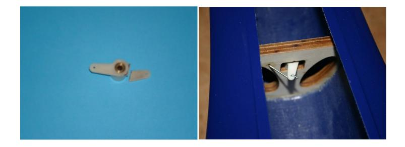
Trim the control horn for the from landing gear leg to make it steareable.install the control horn in the fuselage on the landing gear leg. And install a servo with pushrod.
