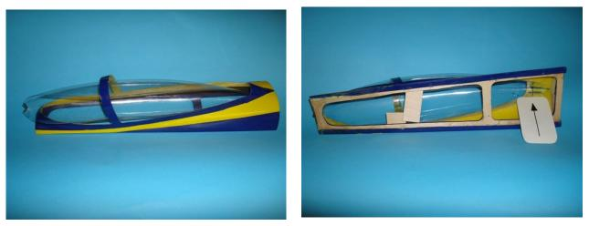
Slide the clear canopy in the frame from the front. Fit and cut the back end as marked in the above picture.
