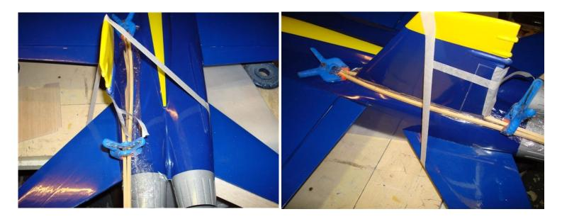
Now it is time to glue the vertical fins in place notice that we use two hardwood sticks and 2 clamps to act like a vice. Use 30 minute epoxy. (sand the inside edges of the fins first before gluing)
