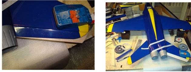
Glue the stabilizers in place with 5 minute epoxy (only apply epoxy in the slots), remove excess epoxy with cleaning alcohol before the epoxy cures. Check if both stabilizers are on the same angle. When you leave the glued parts to settle you can put a small distance block underneath the tips of the stabilizer. Make sure that the distance blocks have the same height.
