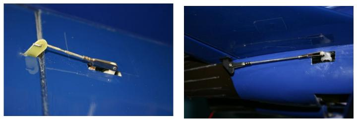
Install the control horns as included in the kit or use your own. Make a Z bens on one side or use 2 clevises on both sides.
