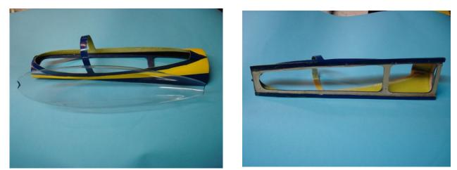
Canopy assembly, trim the edges of the clear abs canopy to size, go slowly you don't want to cut of to much. Sand the plywood frame to size. Trial fit the cockpit frame with Plywood frame on the fuselage. Install the dowel Glue the plywood frame with 5 minute epoxy glue inside the glass fibre frame.
