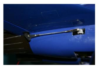
Look at the top right servo for the elevator servo installation. Cut a small slot in the fuselage with a dremel for the servo control horn. Now you can glue the servo in the fuselage with 5 minute epoxy. Cut a small slot for the control horn in the elevator. Trim the top tab of the control horn so that it does not protrude the top surface of the elevator. Glue the control horn in place with 5 minute epoxy. Install the pushrods with clevises as shown. Do this for both sides.
