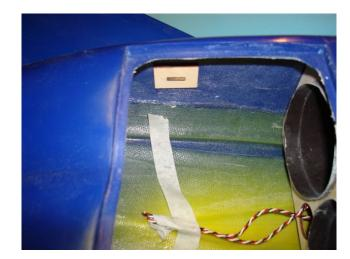
Fit the tube to the fanunit. (read fanuit installation instructions first) You should have installed the motor and ESC already. Make a hole for the wires from the esc and route them trough the just made hole.. Now take of the tube and insert it from the back by squeezing the tube a lilttle. Leave enough room to install the fanunit.
