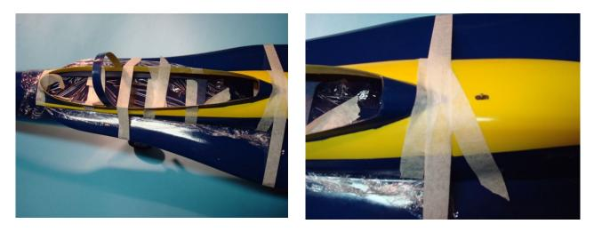
When you glue the plywood frame in place cover the fuselage first with a piece of plastic film. Tape the fibre glass canopy frame to fuselage to get an exact fit.
