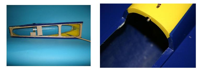
Glue the Clear canopy in the frame with 5 minute epoxy. Install the canopy release.
