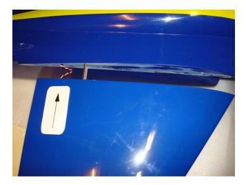
Trial fit the wings to the fuselage. Don't force the wing joiner in the fuselage. Before gluing the wings to fuselage insert an extension leads for the aileron servos . Se above picture. Glue the wings with slow 30 minute epoxy.
