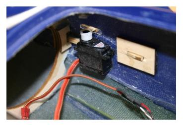
Note the bracket, this bracket must be glued inside the fuselage to support the front dowel of the stabilizer, se left picture. Now fit the elevator to the stabilizer. Now fit the stabilizer with elevator in the slots in the fuselage. Make sure that the elevator can move freely. Before you install the servo make sure the control horn is placed in the middle position. Do this with your radio and receiver.
