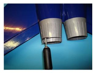
Trim of the ends of the exhaust tubes about 10 mm. Exhausts diameter should be around 58 mm.
