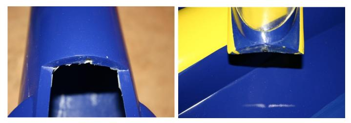
Install the dower in the front of the canopy frame. Make accordingly a hole in the fuselage.
