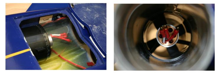
Now install the fanunit. Chamfer the front of the shroud of the fanunit a little with a sharp knife this will make it eassier to install the fanunit inside the duct. Now route the esc wires trhrough the hole in the trust tube you made.. And slide the Trust tube over the back end from the shroud. Use adhesive tape to attach the trust tube to the fan shroud.
