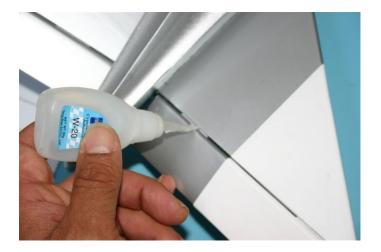
Glue the hinge in place with thin CA glue from the bottom side look at the above picture. In the picture the elevator is shown, but the aileron hinges are glued in the same manner.
