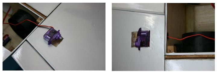
Place your servo ( 2 KG/cm torque minimum) over the pre-cut hole of the wing. Leave room for the control horn of the servo. Adjust the hole for your servo with a X-acto knife . Don't get confused wings from our phantom are shown.
