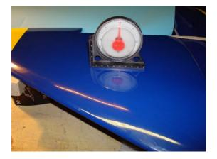
Use tape to keep the wings tight to the fuselage while the epoxy cures. Make sure that the top surface from the wings are level.
