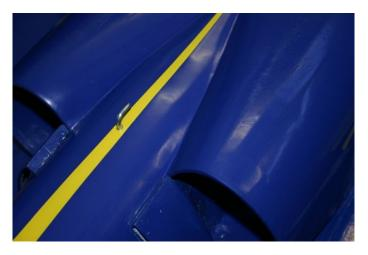
IF You use a bungee you must install the bungee hook, the best location is between the front of the 2 intakes.Glue the first the plywood block 12x30X20 mm in the fuselage then drill the hole for the hook which also need to be glued in place with 5 minute epoxy.
