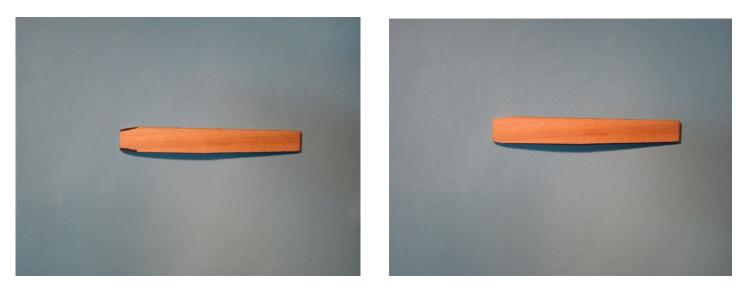
Sand of the inside edges of the wing joiner like in the picture above.
