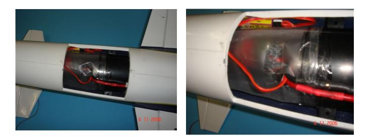
Before you install the fan-unit you must add some tape to the front off the shroud, so that the shroud will fit tight in the intake tube. Also the battery extension wires should be routed first through the fuselage.
