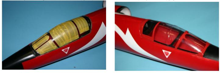
Put masking tape around the frame line on the canopy and spray paint the top. After removing the masking tape your cockpit should look like this.
