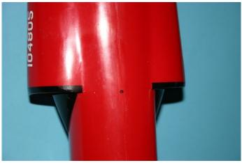
For the installation of the bungee hook you must align a ruler wit the front of the bottom intakes like in the above picture, mark the middle with a marker. This is the bungee hook location.
