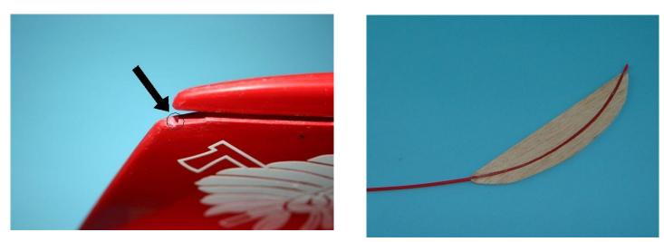
First thing to do is drill a 2.5 mm hole in the back of the top back fin. As you can see in the picture above it's just left above the tomahawk. This is where the pushrod with Bowden-tube should come out. Now glue the red Bowden tube between the 2 supplied balsa pieces with 5 minute epoxy or CA glue. See picture above right.
