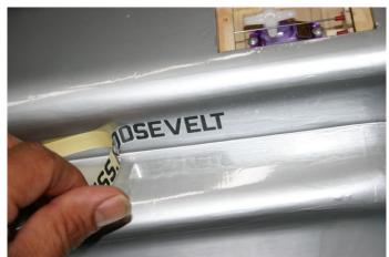
Line out the decal on the area where you want to put the decal. Press the adhesive part. Check if the decal is ligned out and remove the rest of the protective back.
