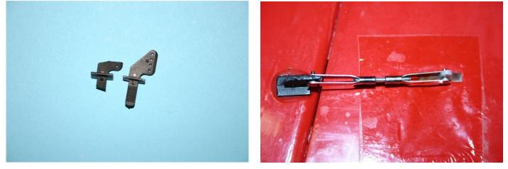
Trim the 2 control-horns for the ailerons as shown in the above picture. Now make a slot in each aileron size as the tab from the control-horn, the slot should be inline with the servo horn. Now glue the control horn in the aileron with 5 minute epoxy. Next step is the actuator arm, Cut off the treaded part from the treaded steel 2mm pushrod . Turn on both ends of the tread a clevis, adjust the length and insert the clevises in the pushrods.
