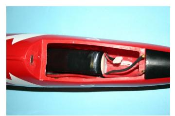
Drill a 2 mm hole at the marked location ( the former from the battery-tray in right under here). Now glue the bungee hook in the hole with 5 minute epoxy. Battery is secured with Velcro in the fuselage. Battery shown is a PQ2500 4S1P
