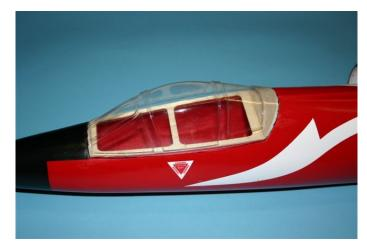
Trim the front, back and bottom edges from the ABS canopy now align it an tape it on the fuselage.
