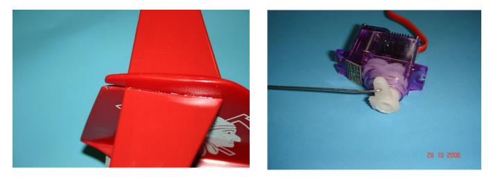
Now glue the stabilizer in the fin with 5 minute epoxy. Remove the excess epoxy with a cloth soaked with cleaning alcohol. After this you must make a Z-bend in the 0.8mm steel push-rod See page 7 how to make Z-bend.
