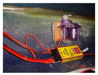
On the left picture you see the 4 channel micro receiver attached next to the servo with Velcro. You can also tape the servo wires to the top. So the wires will not be in the way when you install the ducted fan.
