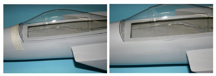
Mark the Outline from the fuselage on the Canopy with a marker. Now trim of the plastic along the marked line. Repeat this step until you have a good fit of the ABS canopy
