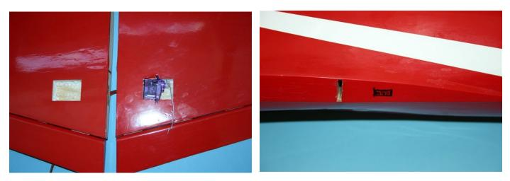
First install the servos in the wings, lengthen the servo cables to 300 mm. mark the hole on the fuselage to route the servo through. Cut out the hole with a dremel tool or use a sharp knife.
