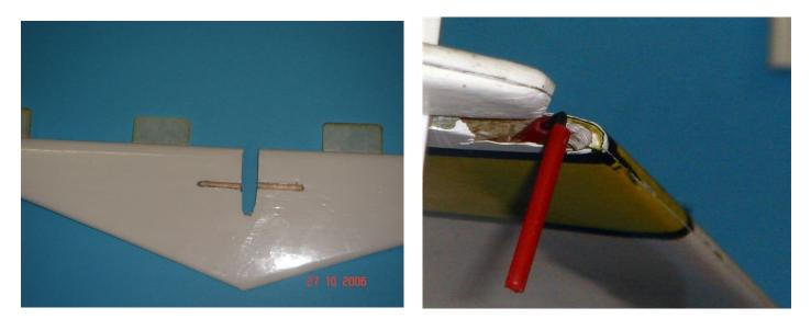
Now make slot on the bottom side of the elevator 2 mm 25mm long only on one side to fit a piece of the red Bowden tube. Make sure your servo is in the middle position. Now bend the steel rod 90 degrees as in the above picture and slide the Bowden tube on.
