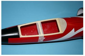
Get the canopy bottom , front and the back plate , place on the fuselage . secure the bottom plate with some tape. Now glue the front and back plate to plywood canopy bottom.
