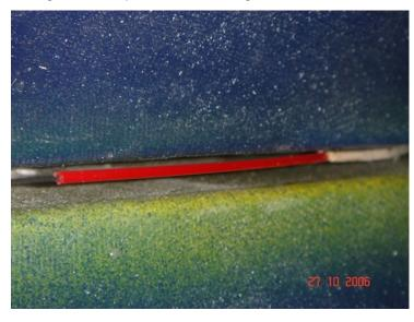
Now glue the Balsa bracket with the Bowdentube inside the fin with 5 minute epoxy, glue it to one side of the fin. The red Bowden tube should come out the fin and should be trimmed flush with the slot-edge inside the fuselage the Bowden tube and 0.8 mm steel tube should run parallel with the fuselage top surface
