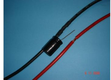
The wires from the ESCs need to be extended all the way to the front. Use at least 4mm2 wires. Because of the length we advise to put in the middle of the extension wire 1 or 2 capacitors e.g. 470 uf 40V. Strip some of the insulation of wire and solder the capacitor(s) to the wires, than insulate with shrink tube.
