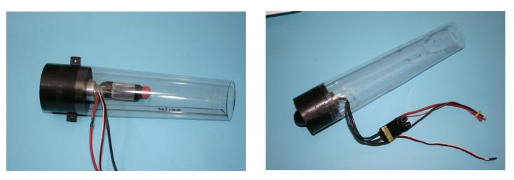
Read the installation instruction from your fan-unit first. Install motor and ESC first. You can either install the ESC inside the thrust tube or outside. We recommend to place the ESC behind the motor inside the thrust tube.
