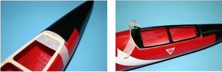
Drill a 3 mm hole trough the front plate and fuselage. Let the dowel stick out a couple of mm and glue the dowel to the plywood front former. Remove canopy frame from the fuselage. Now sand the edges of the canopy frame so that it fits within the outlines of the fuselage.
