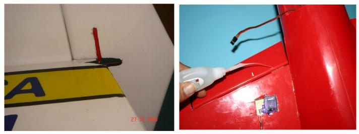
Now install the elevator Glue the Bowden tube ( see above picture ) in the stabilizer with CA glue . make sure the elevator is in it's neutral position. Now you can fixate (glue) all the hinges form the elevator and ailerons in place. Do this from the bottom side , use thin CA.
