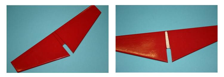
Now we are going to install the elevator, mark the outline of the fin on the elevator as in the above picture. Than trim inside the marked lines the covering and remove it .
