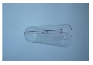
Cut out the unrolled surface for both trust tubes. Put the ovelap area inside. Roll the pvc to a tube and apply outside adhesive tape. The Edge should match the innerline of the overlap area. Now you have a perfect conical trust tube.
