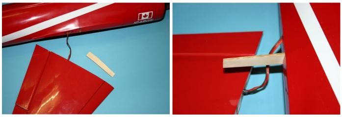
Fit the hardwood wing joiner in the fuselage and wing and see if the wing fist nicely. Sand the fuselage root first .
