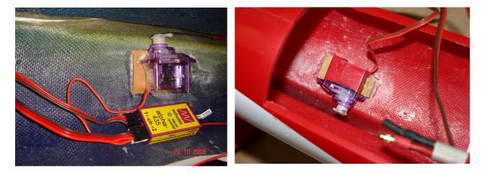
Here you see how the servo is mounted (glued) servo should be taped in or put in a heat shrink tube and then glued on the plywood tray, or glued between two plywood blocks 6x6x 10 mm.
