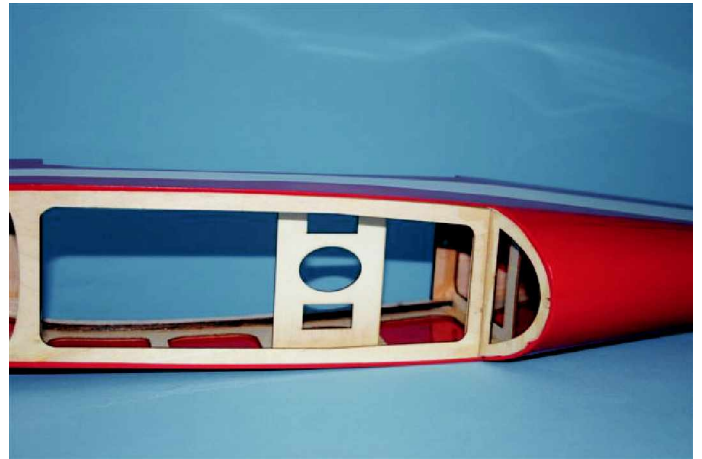
Servo- tray shown for rudder and elevator servo.
