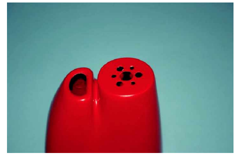
Use a dremel or a drill to make the holes.
