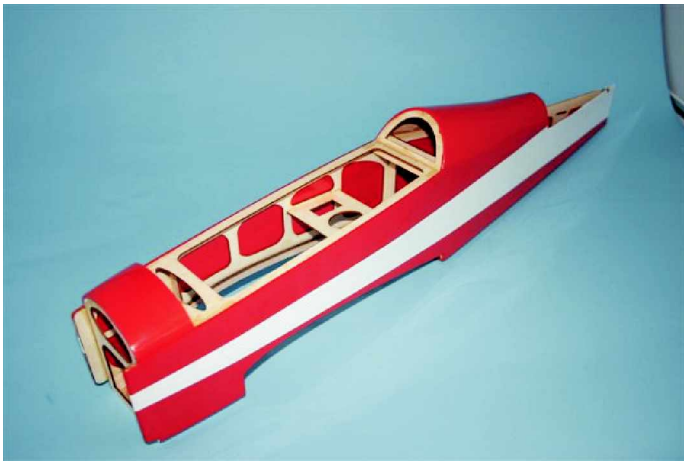
Fuselage is made of liteply and balsa
